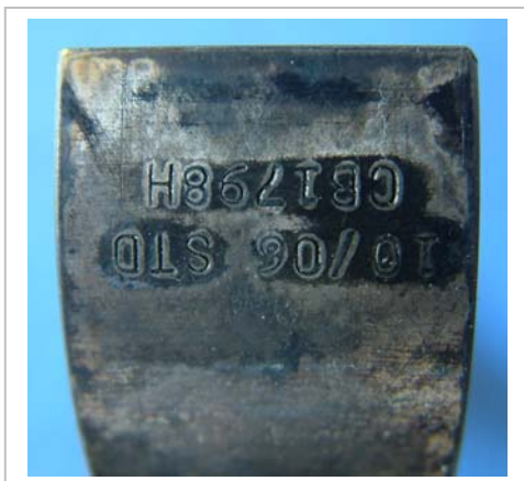
Used bearing shows how heavy stamping disrupts the back contact
